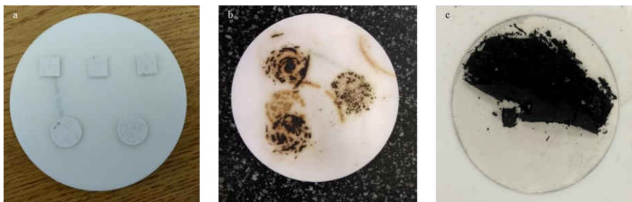
Figure 42. The 3D printed composite samples after sintering: a. PVA- \text{Al}_2\text{O}_3 ; b. PVA-LSM; c. PA12-LSM.
