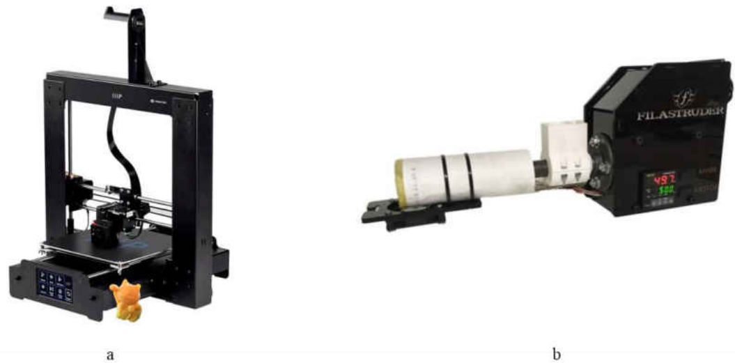
Figure 36. FDM devices: a. 3D printer; b. extruder.
