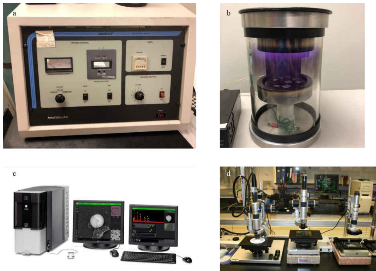
Figure 46. Inspection equipment: a. sputter coater; b. sputtering process; c. SEM; d. optical microscope.
